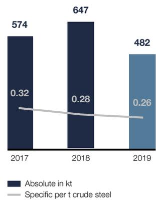
**NO<sub>x</sub> emissions** of all crude steel producing production sites in t/in kg per t of crude steel produced
